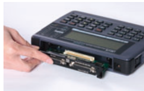
▲New communications standards different in hardware specification are supported with the replacement of the measurement board.
