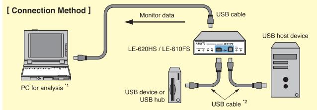
\*1 It is recommended to install the provided analysis software to a PC model incorporating a high-speed USB 2.0 port. If a full-speed USB port is used, however, data recording only to the built-in memory of the analyzer will be guaranteed. If the USB host used for measurement is a PC model supporting the operating conditions of the analyzer, the PC model can be used for analysis purposes as well.
