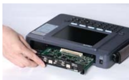
▲ Differing communications standards are supported by simply exchanging the measurement board.
