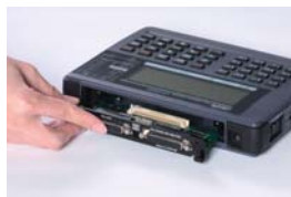
▲ New communications standards different in hardware specification are supported with the replacement of the measurement board.
