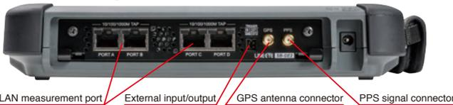
LAN measurement port External input/output GPS antenna connector PPS signal connector
