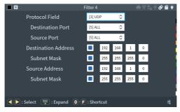
It is configured by filter 4 to monitor only the frames of UDP protocol which have "192.168.1" for the network address part of both source IP and destination IP.
